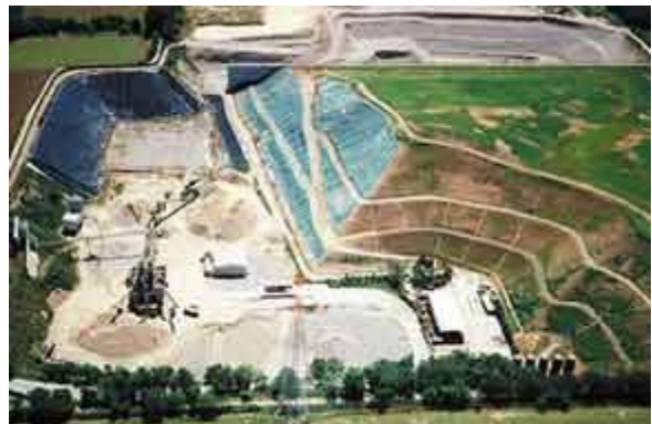
Cerro Maggiore (Italy) Aerial view of the final closure of the municipal solid waste landfill
